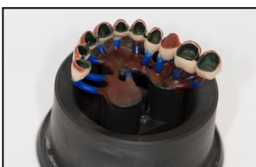
Fig. D Spruing technique from bird eye view- pistons need to
